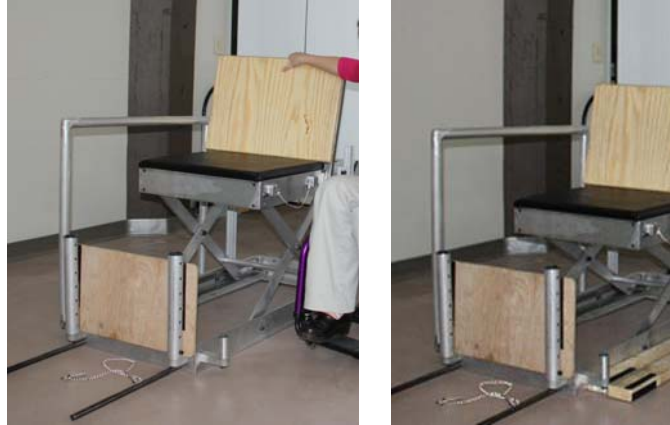
Height adjusted and spacers added at floor level
